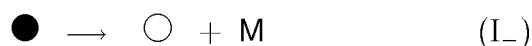
FIG. 1. The reactions at the basis of the Langmuir theory: adsorption is seen as the formation of filled surface sites (denoted with \bullet ) by the reaction of empty surface sites (denoted with \circ ) with gas-phase molecules M , while desorption is regarded as the reverse process.
